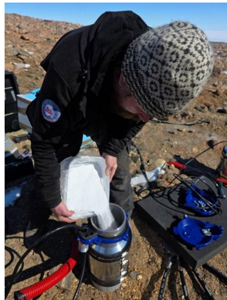
Preparation of the borehole casings for hosting the seismic sensors (left). Filling the casings with sand for insulation after installing the seismic sensors (right). Photo: NORSAR.
