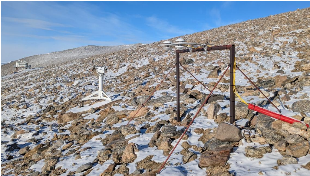
Reinstalled broadband radiation sensors for monitoring the surface energy budget. Photo: NPI/U Leeds.
