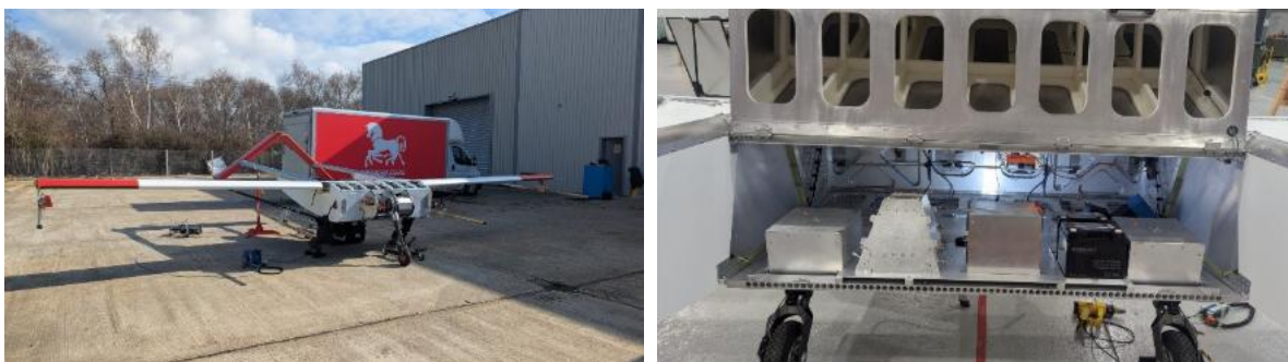
Left: TONe-RPAS under production in Southampton. The VHF radar antennas can be seen under the wings. Right: Radar hardware installation in the fuselage. Photos: Andreas Tøllefsen, NORCE.
