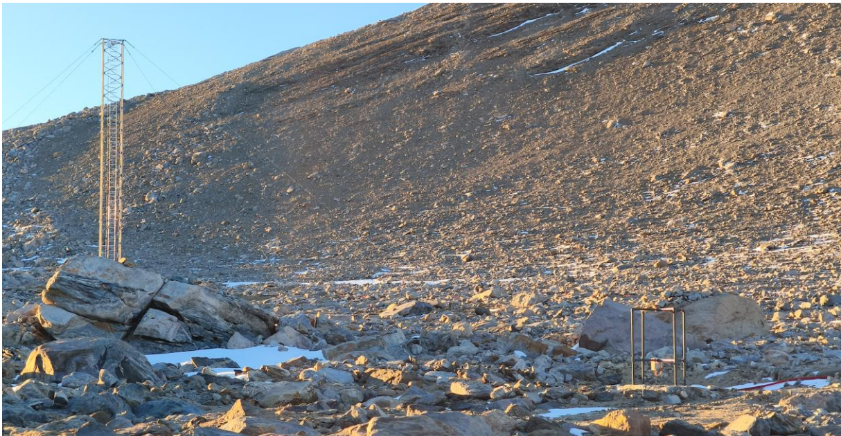
Part of the ionosonde system – the transmitter antenna and one of the receivers antennas - at Troll Research Station in December 2025. Photo: W. Miloch, University of Oslo.
