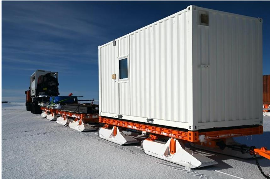
*The UiO instrument container arrived in the middle of January 2025 by ship and was transported to the station on sledges from the coast. Photo: Wojciech Miloch, UiO.*
