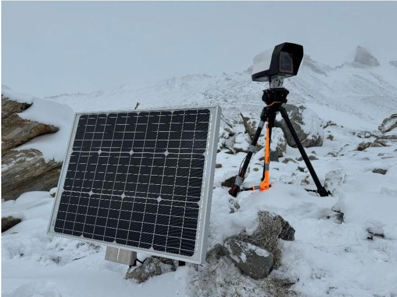
*Time-lapse camera with 4G connection installed on Trollhaugen for monitoring snow petrels. Photo: Sebastien Descamps, NPI.*
