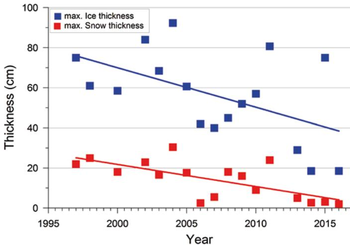
**Fig. 4.5** Maximum seasonal sea-ice and snow thickness (cm) in inner Kongsfjorden 1997–2016. Lines show the linear trends: blue – ice-thickness changes (–24.7% per decade) and red – snow-thickness changes (–41.7% per decade). There were no *in situ* measurements in the years 1999 and 2001 because regular monitoring started first in 2003, and none in 2012 because of little ice. Observations from 1997, 1998, 2000 and 2002 were made in connection with research projects
