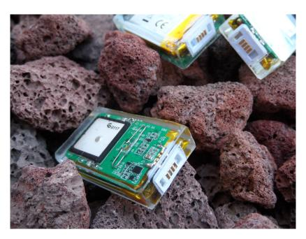
Other than devices in ThermoSeal, which are hermetically sealed, Potted devices have their interface exposed to the environment. This requires a different type of connector.
