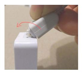
Even though the connector is Gold plated you need to protect the interface against corrosion especially if you are going to use it in salt water. Some use wax or dip-in-rubber. A coat of latex color, applied only to the terminals would be an alternative choice, this can be removed with rubbing alcohol.
