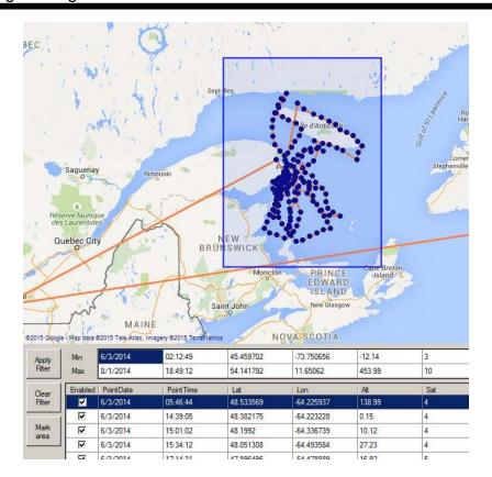
The spatial filter becomes effective after the button "Apply Filter" is pressed. To remove the area selection simply right click on the map.
