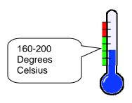
Next step is to adjust the heatgun. The optimal temperature range is 160-200 degrees Celsius (320 – 390 Fahrenheit). If you have an unregulated heatgun you will need to vary the distance between air outlet and device to not overheat the material. You may also want to shield the battery. The battery may get damaged by too high temperatures.
