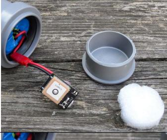
GPS is located in the cap, remove the foam spacer.
