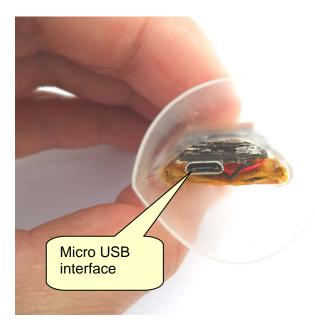
Some device versions have different interface connectors. Especially devices potted in Epoxy resin will feature a special connector that has some critical points that need to be considered. Please see section "Enclosure Variants" for important information.
