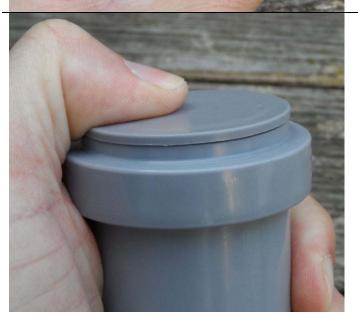
Push cap slowly into the tube, check that bottom cap is also all the way pushed in.
