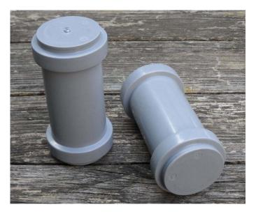
One cap contains the GPS receiver, while the other end has a small hole closed by a screw. This is the air purge hole and needs to be open while opening or closing the enclosure. Otherwise air pressure in the enclosure will either prevent removing a cap or the cap cannot reliable closed.
