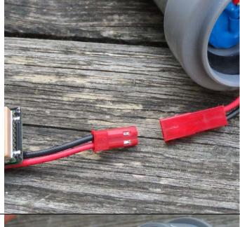
The GPS can get disconnected from battery to charge the battery with high current charger.
