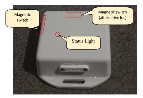
The device uses a waterproof magnetic interface connector. There are some things to consider with this interface type:
