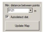
The value of minimum distance tells the program that all points with a distance lower than the defined value will be filtered out. The value can be selected manually or automatically based on the map scale. Button "Update Map" needs to be pressed each time the value was changed manually or the map was zoomed in/out.
