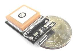
Used in thousands of GPS tags around the world CatLog became the standard GPS data recorder for wildlife bio-tagging. The device will record the position in an adjustable time interval. The movement profile can later be displayed on a map or exported to use with other software.
